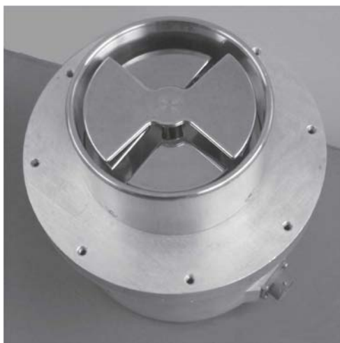
Figure A1-3. Photo of the sensing electrodes in a field mill
