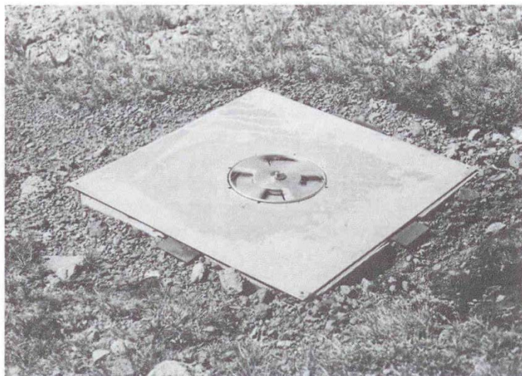
Figure A1-4. A flush-mounted field mill for calibration
