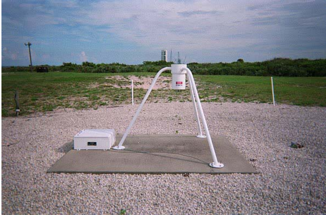
Figure A1-5. Photograph of a field mill in the LPLWS
