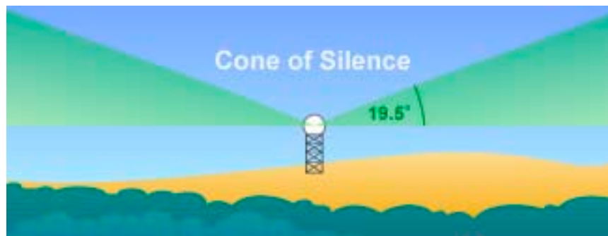
Figure 1. Cone of Silence for WSR-88D 'NEXRAD' radar systems
