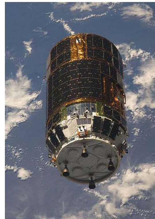
HII Transfer Vehicle (HTV) ~117 volt solar arrays Dock: 17 Sept 2009 22:26 UT
