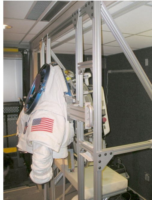
Figure 12.—Upper torso of I-Suit with Cryopac.
