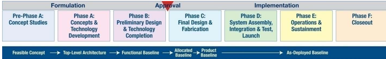
Figure 3. NASA program/project lifecycle phases and stages (SP-6102).
