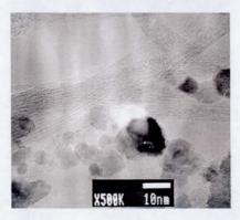
545 °C: even less nontubular impurities, metal particles starting to lose graphitic coating
