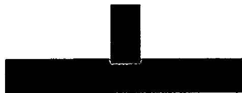
6: Etch Substrate around Cavity
