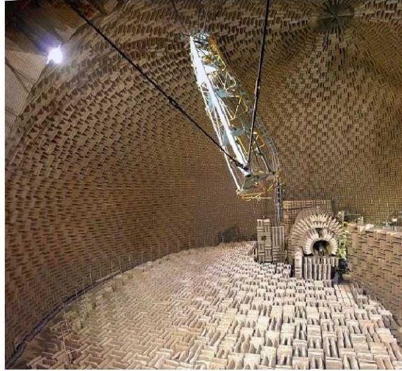
Fig. 3 The AeroAcoustic Propulsion Laboratory with dual flow jet exit rig in the NASA Glenn Research Center.
