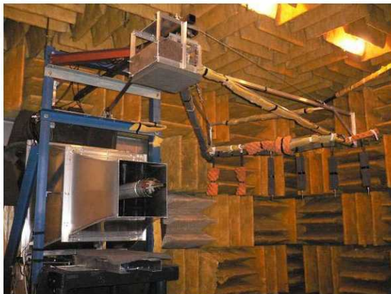
Fig. 1 The Pennsylvania State University high speed jet noise facility a) schematic b) photograph.
