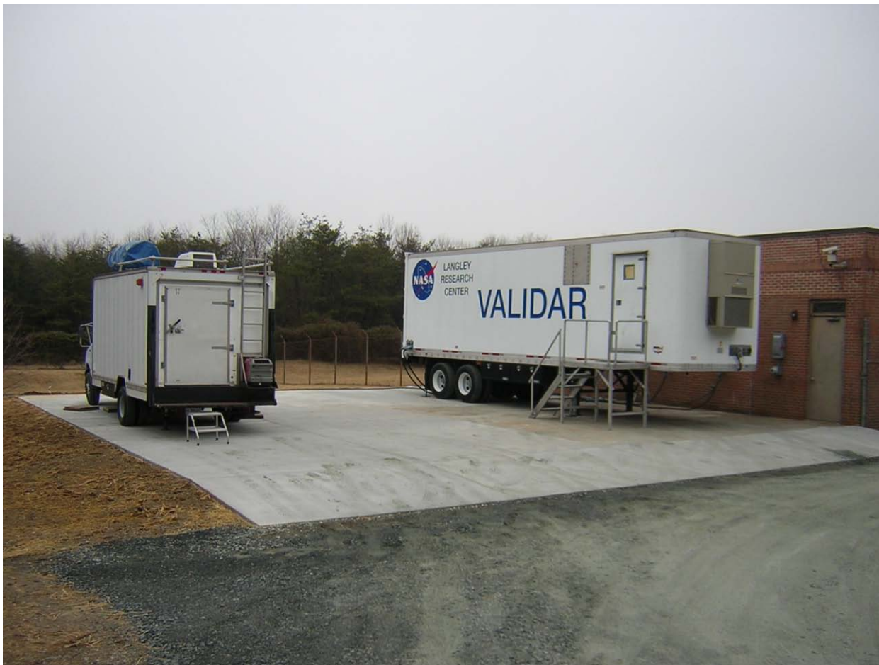
Fig. 9. Photograph of field test site at the Howard University Research Campus in Beltsville, Maryland. The 2- \mu m lidar is housed within a 35-foot long trailer testbed called VALIDAR. The other trailer houses the Goddard Lidar Observatory for Wind.
