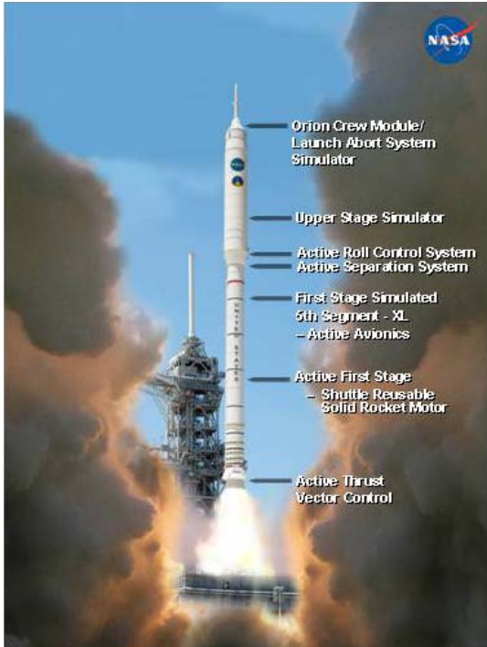
Figure 2. The Ares I-X Flight Test Vehicle incorporates both flight-like and mass simulator hardware.
