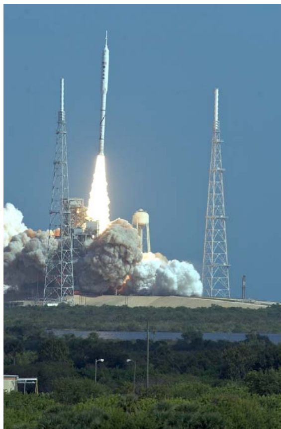
Figure 1. The Ares I-X fly-away maneuver angles the flight test vehicle away from Launch Complex 39B.
