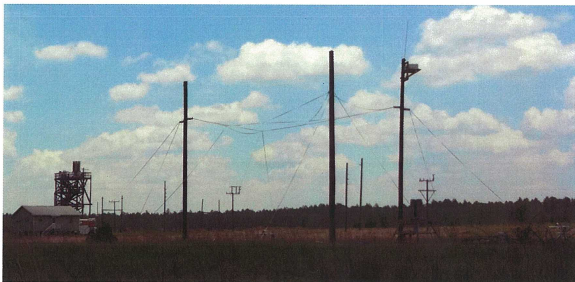
Figure 1. Scaled-down model of the lightning protection system of Launch Complex 39B, built at the ICLRT, Camp Blanding, FL.
