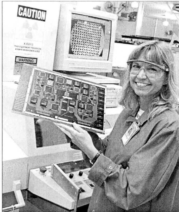
Lab technician holding a test board consisting of lead-free electrical components and solder
