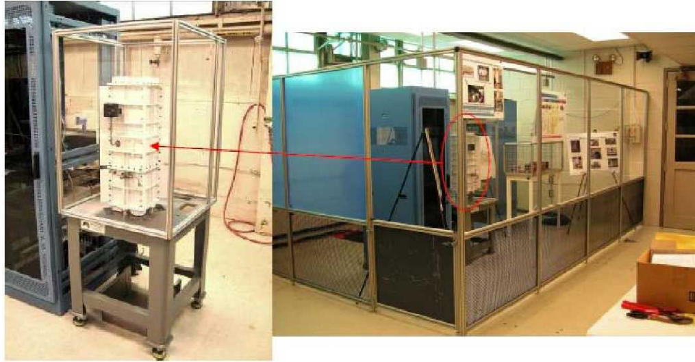
a) ASRG EU in enclosure on test stand b) ASRG EU and ASC-E #1 and #4 test facility
