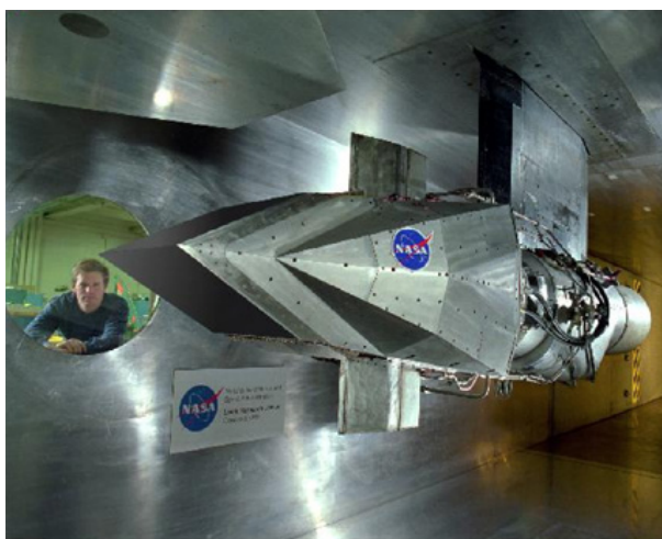
Figure 2. 2DB supersonic inlet attached to J-85 engine in NASA Glenn Research Center 10x10 supersonic wind tunnel. 12
