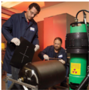
NASA White Sands Test Facility technicians perform radiographic inspection on a filament wound pressure vessel.
