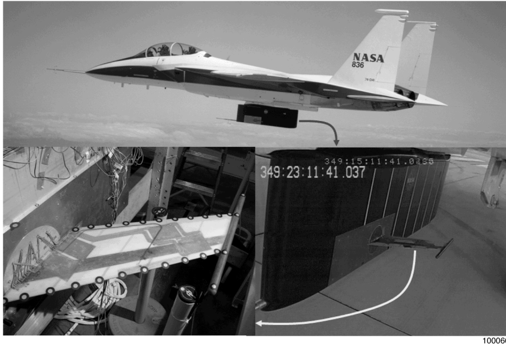
Figure 3. Aerostructures test wing 2.
