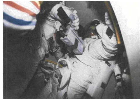
Figure 31.1.2.12 – Hydrazine monitor being used in the airlock following an EVA
