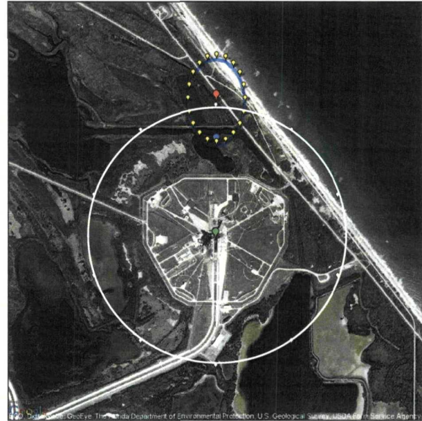
Figure 6. Google Maps visualization of a lightning uncertainty ellipse overlaid on the radius around the POI with a semi-major axis heading of 180° as graphed in Figure 5.
