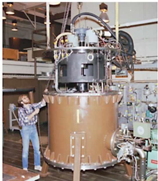
Figure 2.—Test article lowered into dynamic spin rig.
