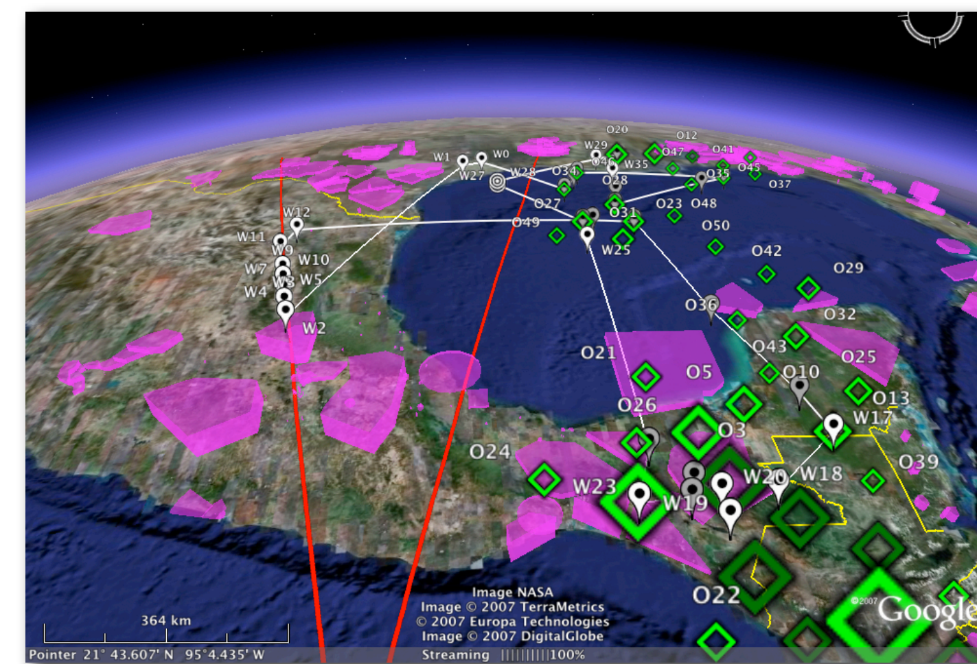
Collaboration: Results of automated data mining and flight planning visualization ported to KML and viewed in Google Earth. Right: Special use air spaces (magenta), observation points (green), satellite ground track (red), and plan (white). Below: Close up of plan showing spiral leg and waypoint detail.
