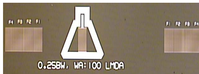
Figure 1. SAW strain sensor comprised of an interdigitated transducer (IDT), and two banks of four OFC reflectors on a Langasite substrate.
