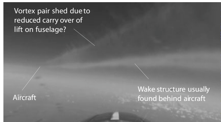
Fig. 1 Frame from motion picture taken as side view of condensation wake of aircraft at cruise altitude indicating that one part of the vortex wake is nearly horizontal, as expected, and that another part is moving rapidly upward [7].
