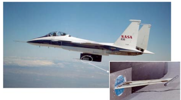
Fig. 1. The aerostructures test wing mounted on the NF-15B for flight flutter testing.
