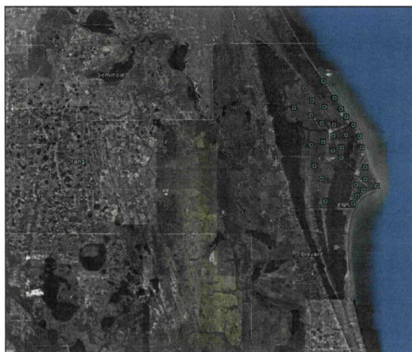
Figure 3. Map of the 31 surface electric field mills in the Launch Pad Lightning Warning System.
