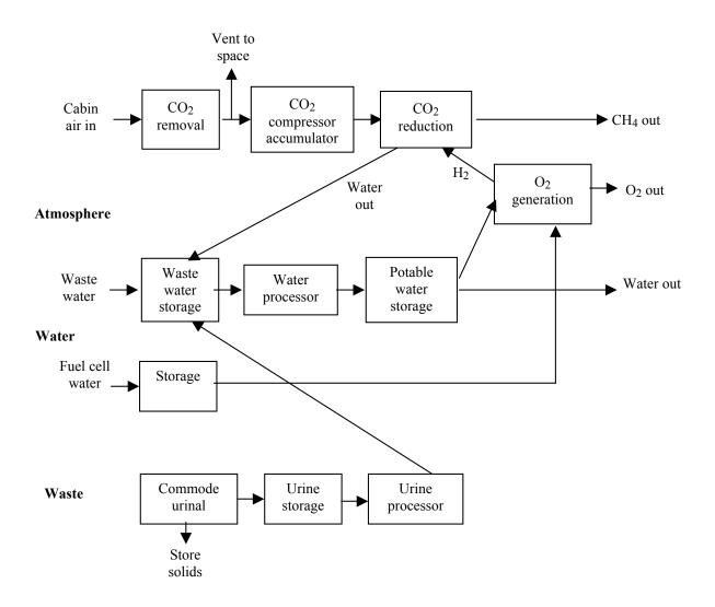
As shown in Figure 1, the ISS life support system contains atmosphere, water, and waste processors. The four bed molecular sieve (4BMS) carbon dioxide removal system is designed to allow the carbon dioxide to be vented to space or to be delivered to the Sabatier carbon dioxide reduction system. The electrolysis oxygen generator provides oxygen directly to the cabin atmosphere. The hydrogen can be vented overboard or used for carbon dioxide reduction.
