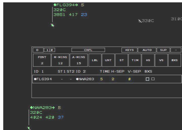
Fig. 13 Two aircraft in conflict, FLG394 (top, southwest bound), and NWA283 (bottom, northwest bound), showing conflict probe numbers in the upper right of their FDB. The conflict list is also displayed.
