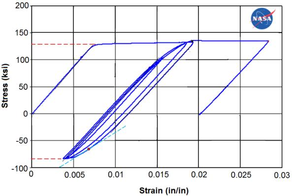
Material response in tension differs than in compression. Bauschinger effect becomes key in developing instability wherein extensive prior yielding in tension reduces the magnitude of the yield threshold in compression by 30 to 40% compared to the virgin annealed state of the titanium.
