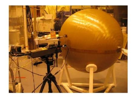
Instead of estimating the stress from the change in tank volume, hypothesis is to measure the strain using a Raman Spectrometer on the exterior of the tank and correlate to stress through the thickness of the overwrap. (Nobel Prize 1930)
