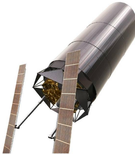
Figure 4: ATLAST-8m exterior view showing twin gimbaled solar arrays.
