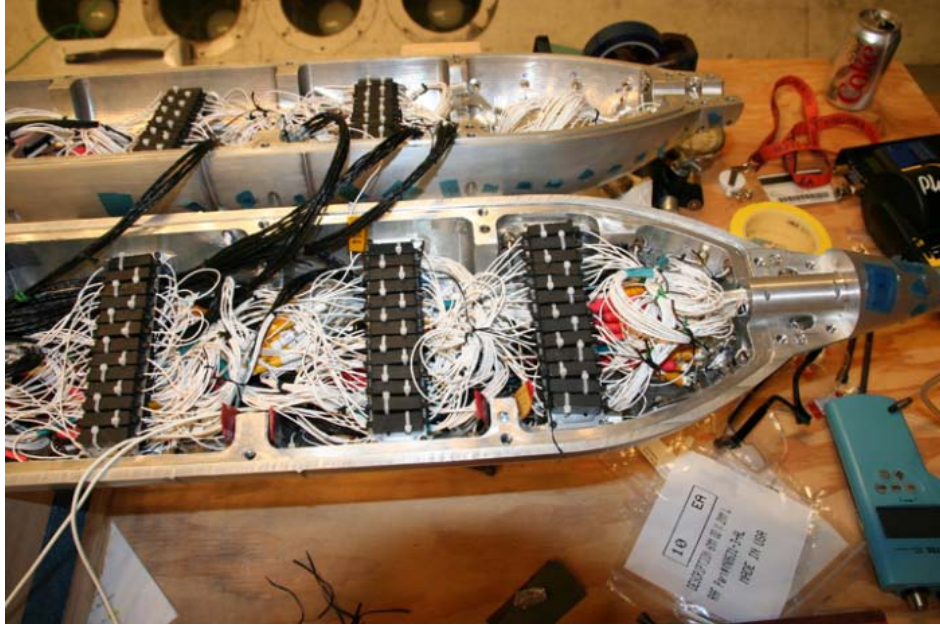
Figure 6. Ares I RBM unsteady pressure instrumentation installation.
