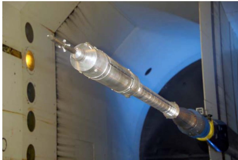
Figure 2. Ares I-X Rigid Buffet Model in TDT (close-up).
