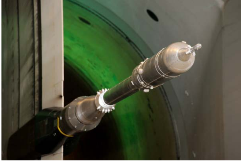
Figure 3. Ares I Rigid Buffet Model in TDT (close-up).
