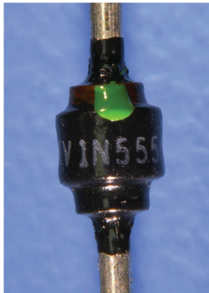
Figure 1. The Keyence VHX-600 optical microscope was used to collect this magnified image of a 1N5550 diode.
