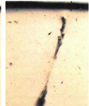
Self healing occurring in repair film in seconds after damage from left to right
