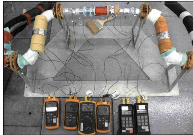
AeroPlastic demo testing on cryo-piping system
