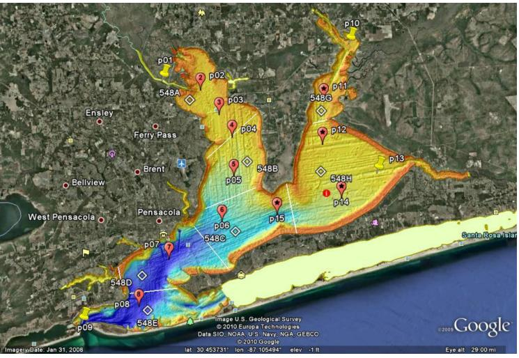
Pensacola Bay divided into WBIDs (548A-H, white line boundaries) with EPA sampling stations (marking pins). Color is bathymetry - shallow in red and deep in blue.
