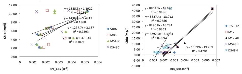
Chla vs. Rrs\_645 at two different stations using small window and WBID scale averages RELEASED - Printed documents may be obsolete; validate prior to use. Needs Assessment for the Use of NASA Remote Sensing Data for Regulatory Water Quality 11
