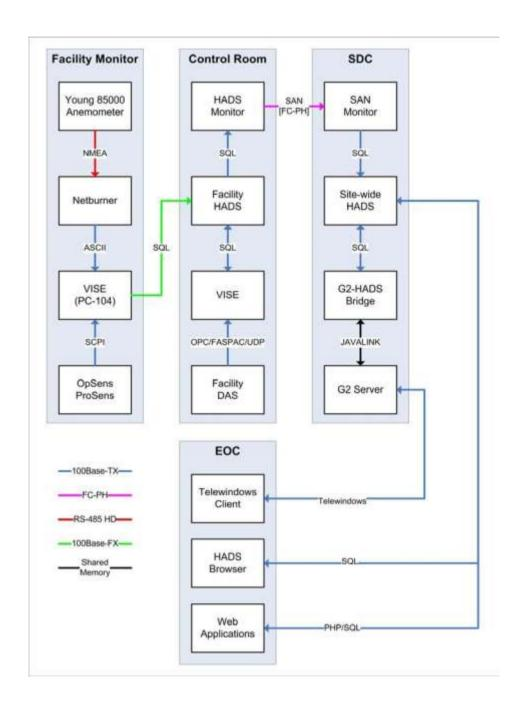
Figure 3. Structural and Wind Measurement Systems
