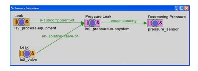
Component Objects: Component objects have the following attributes: anomalies and component electronic data sheet (CEDS). CEDS are uploaded from the HADS and can be displayed at any time. This provides immediate access to component specifications. Component objects in the DM's include valves, pipes, tanks, etc.
