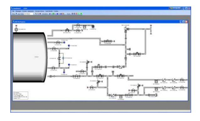
DM's include windows that display warnings and fault conditions that the ISHM-DM detects (Figure 6). Warnings and faults are associated with elements in the DM. Clicking on an element associated with a warning or fault takes the user to the element in a window showing a detailed DM of the subsystem where the element is located.
