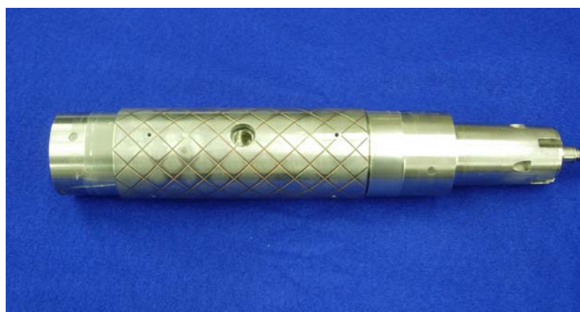
Fig. 2 NASA's MC60D strain-gage balance (photo courtesy of Triumph/Force Measurement Systems).
