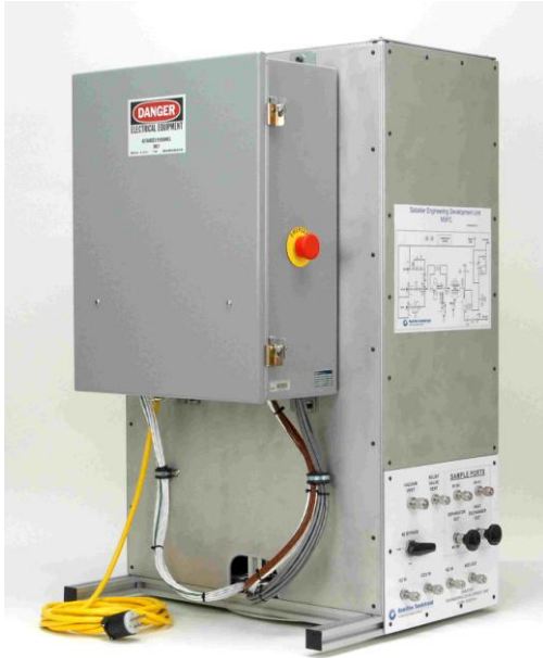
Figure 1. Sabatier Development Unit. The SDU was built as a development model for state-of-the-art CRA technology by Hamilton Sundstrand.
