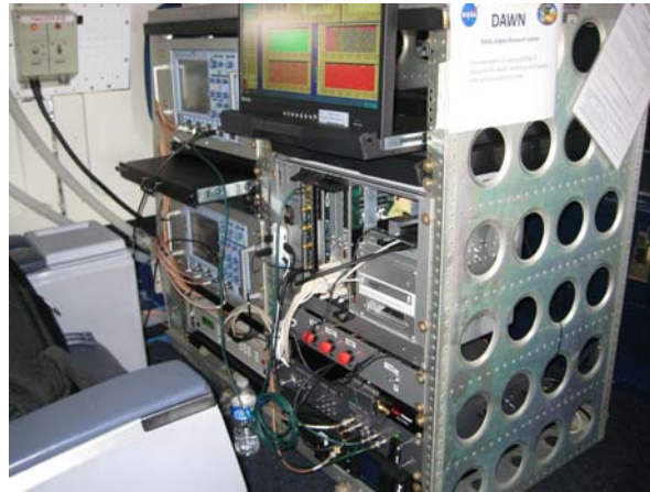
Fig. 5. The DAPDS and the laser electronics system in the DC-8 during the mission GRIP
