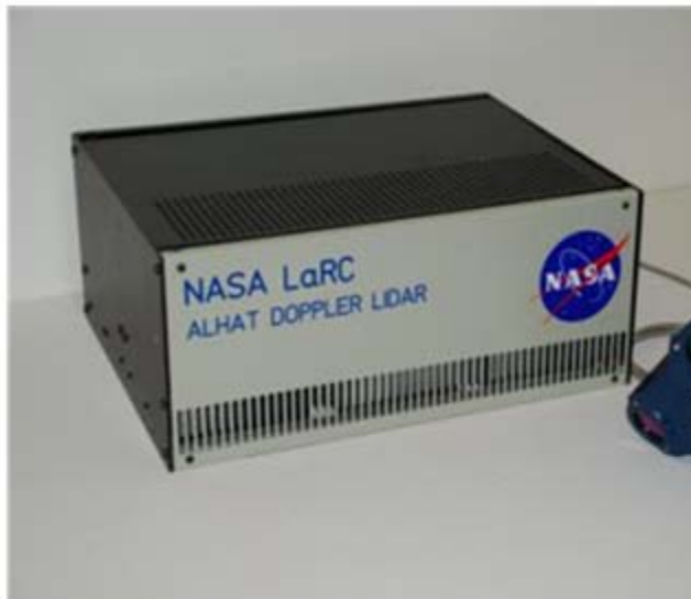
Fig. 3. Doppler Lidar prototype system with a fiber-coupled optical head having 3 lenses pointing to different directions. The Doppler Lidar provides vehicle vector velocity and altitude.
