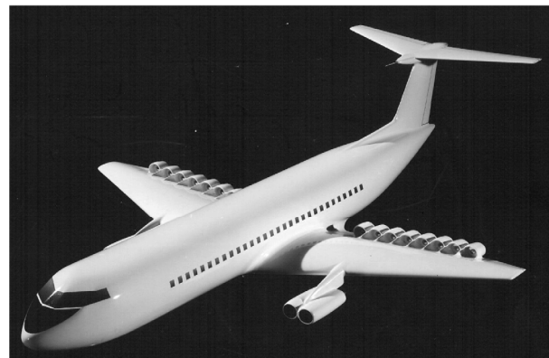
Fig. 6. Short take-off and landing STOL transport using low compressor discharge tip-driven multi-fans [8].
