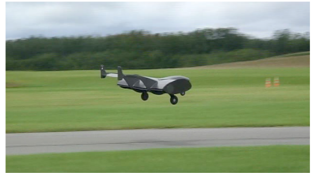
Fig. 3. A cross-flow fan (CFF) unmanned aerial vehicle (UAV) model in flight [5].
