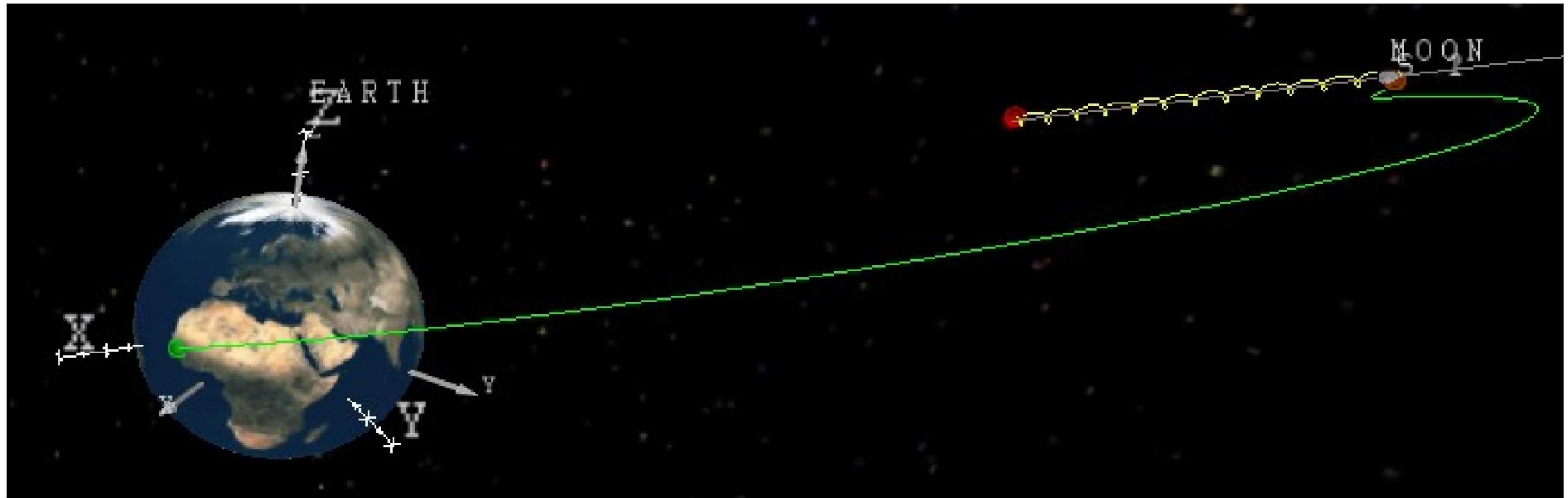
Trans-Lunar Cruise/Coast Trajectory (Earth-fixed frame, Copernicus Trajectory Tool)
