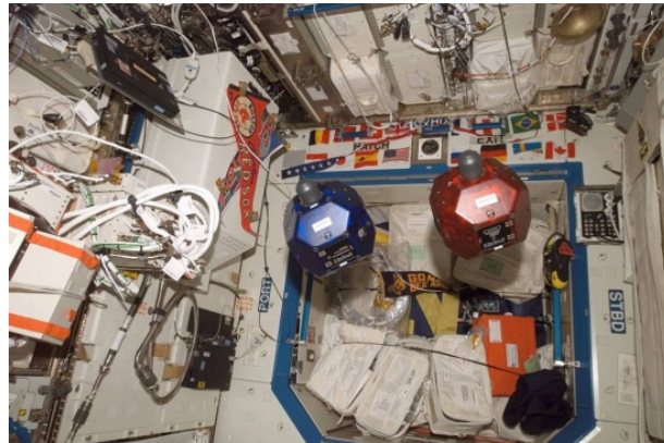
Fig. 2: The SPHERES internal satellites flying inside the ISS under the control of student developed software
