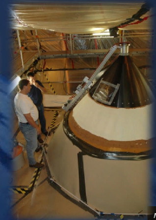
LO 2 Forward Ogive Area (pencil sharpened area)
