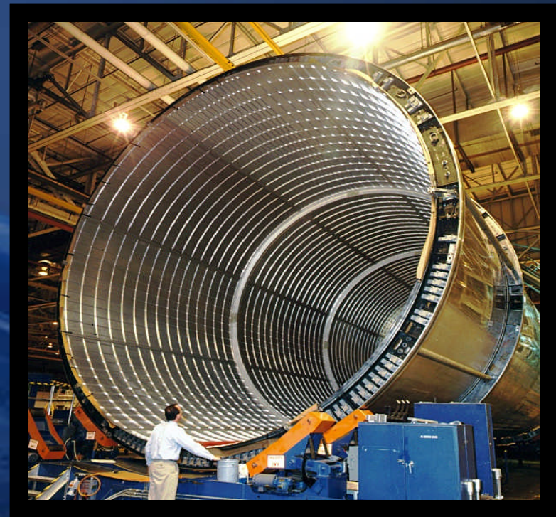
Super Lightweight (SLWT) – Al 2195 alloy
