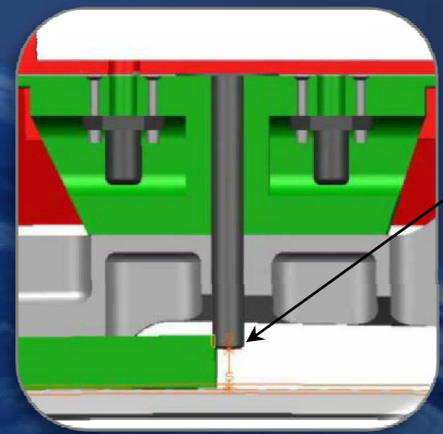
Cryopumping path along shear pin hole eliminated – Issue identified through ET-120 dissections and testing
