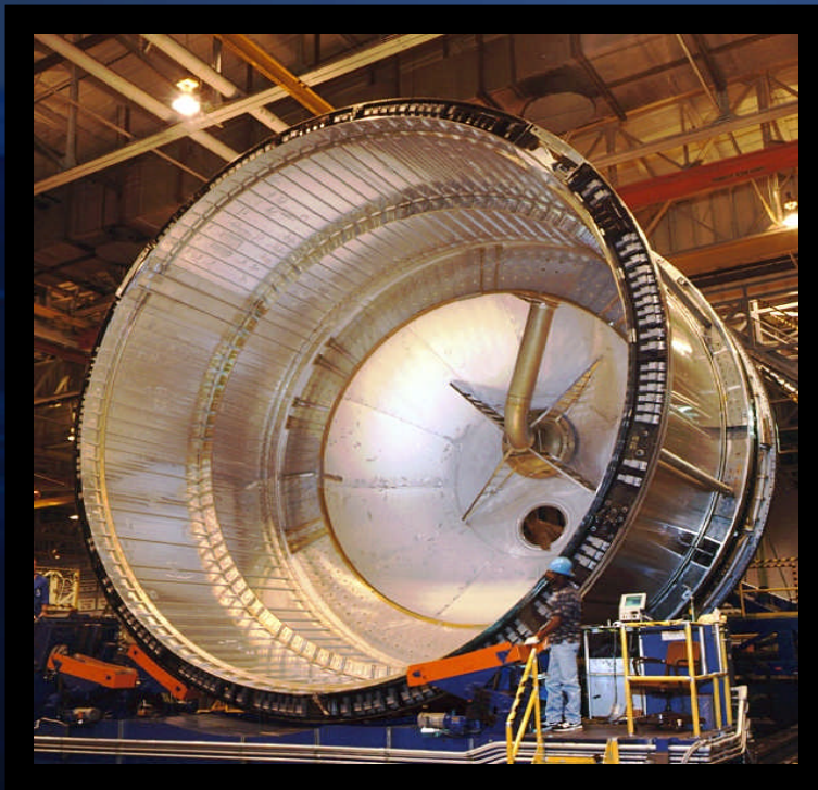
Standard Weight (SWT) and Lightweight (LWT) – Al 2219 alloy
