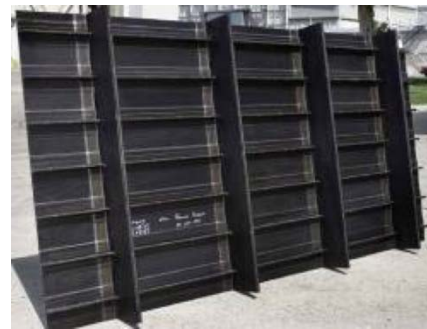
Figure 1. Intersection of PRSEUS stiffeners. Figure 2. Typical PRSEUS panel.
