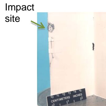
Figure 9. Impact damage site for blade-stiffened specimens.
