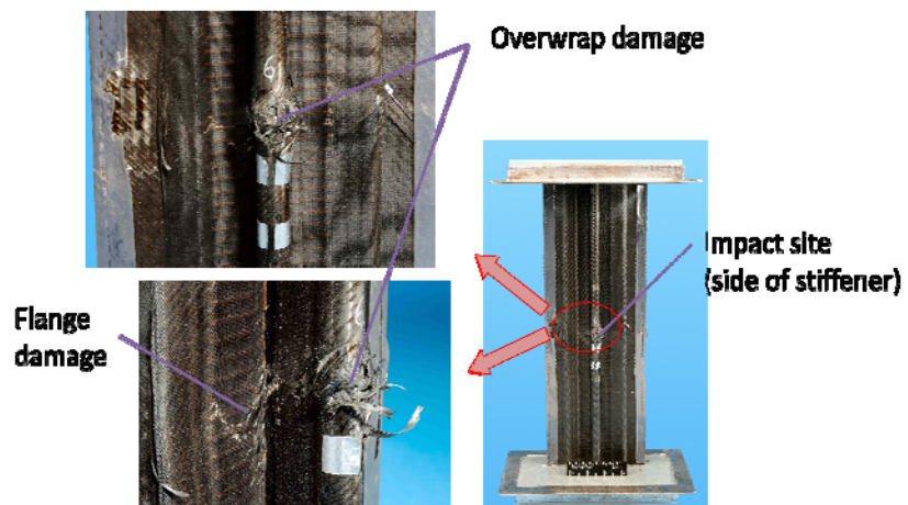
Figure 35. Failed specimen with side impact and no fatigue.
