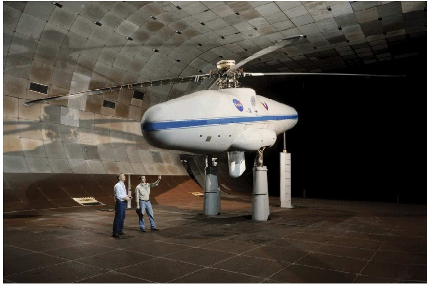
Fig. 1: UH-60A rotor system installed on the Large Rotor Test Apparatus in the NFAC 40-by 80-Foot Wind Tunnel.
