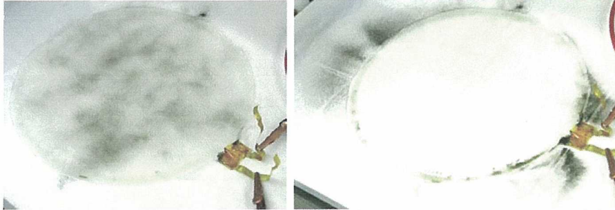
Figure 7. Photographs of the 20-cm diameter transparent EDS for the PEM viewport during laboratory tests. JSC-1A simulant dust was deposited in a relatively uniform fashion, as shown on the left. The photograph on the right shows the EDS after activation. Dust has been removed to the region outside the electrode grid. These tests were performed with the EDS sitting horizontally in a glove box.
