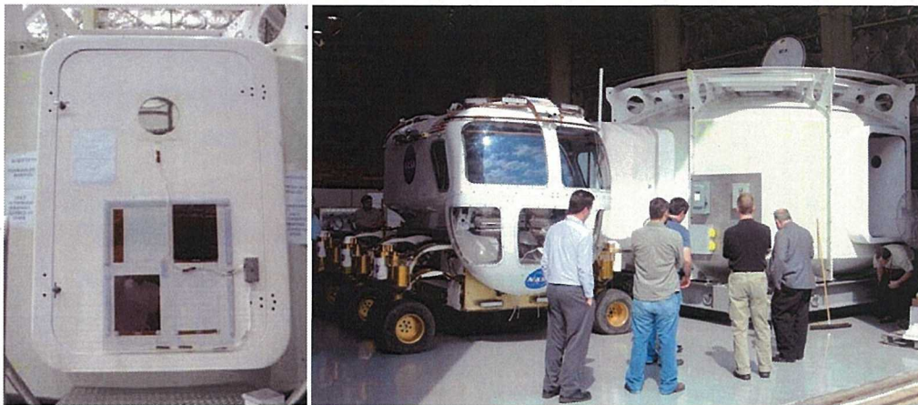
Figure 5 (a). One of the PEM doors with the EDS systems installed. (b) The Lunar Electric Rover mated to the PEM.
