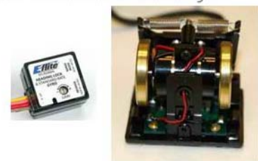
Figure 5. Solid state versus mechanical gyro comparison. Solid state components offer drastically lower cost and size, while offering dramatically improved reliability and accuracy.
