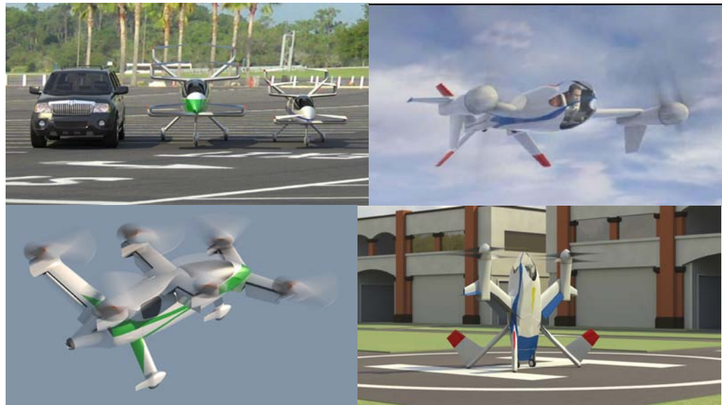
Figure 6. Examples of recently developed advanced concepts that utilize primary electric propulsion. The Puffin concept on the right is a single person tail-sitter VTOL aircraft, while the Samarai on the right is a two person stopped multi mono- rotor aircraft.
