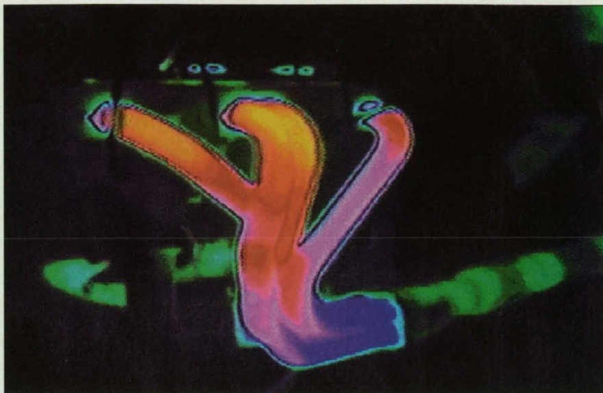
A pseudocolor thermal image of the exhaust manifolds of one side of an automobile engine, captured with FLIR Systems' equipment, showing heat-affected zones during operation.
