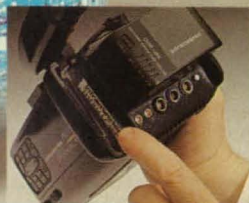
Digital storage of 12-bit images on a PCMCIA memory card eliminates floppy disks. Just plug the card into your PC for image processing and report generation.
