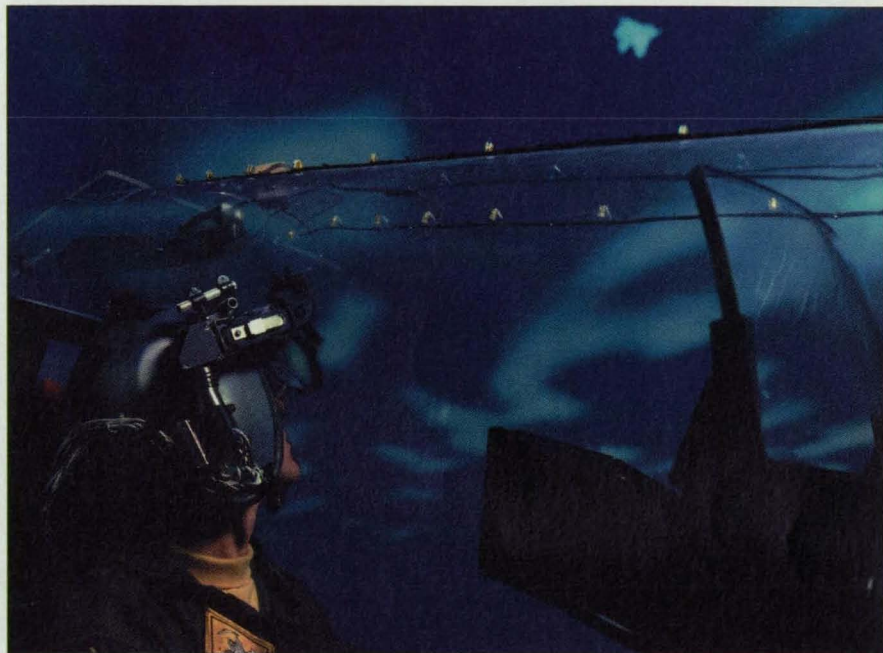
Langley's Differential Maneuvering Simulator incorporates helmet-mounted display technology to simulate air-to-air combat. The simulator has two 40-foot diameter projection spheres with a cockpit in each. Wide-angle projection systems in each sphere present Earth scenes, sky scenes, and images of additional aircraft to the pilot.
