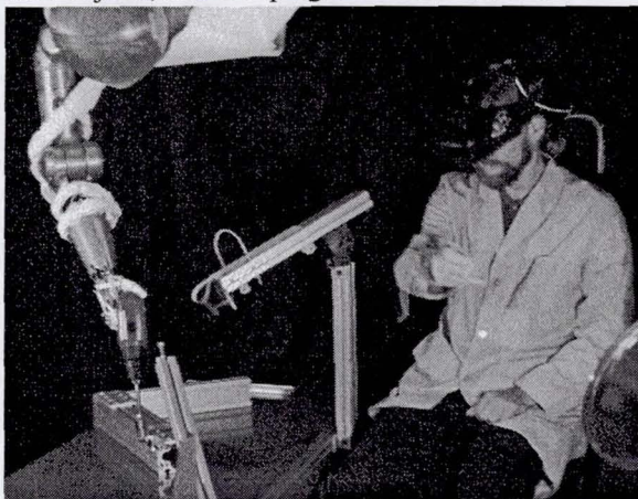
Figure 16 Robonaut using Torque Drill on Bolt
