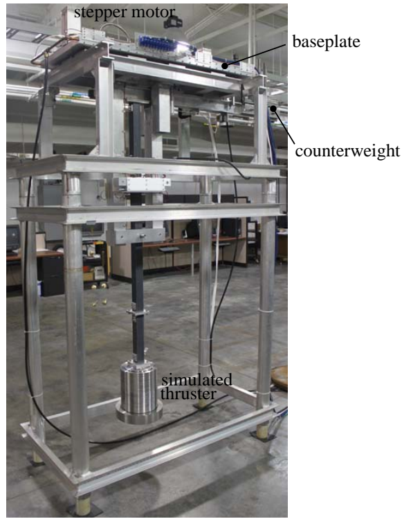
Figure 1. Photograph of the VTS, mounted on a support structure.
