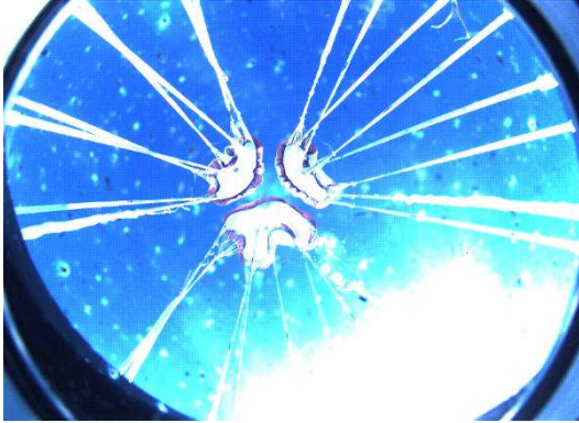
Figure 6b. High-speed cameras captured the severing of the main parachute line.
