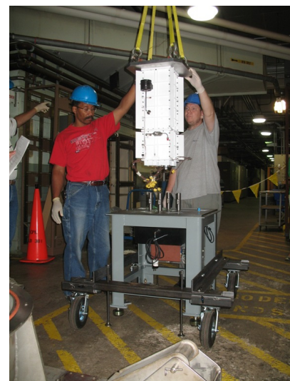
Figure 4.—Test stand transporting the ASRG EU.
