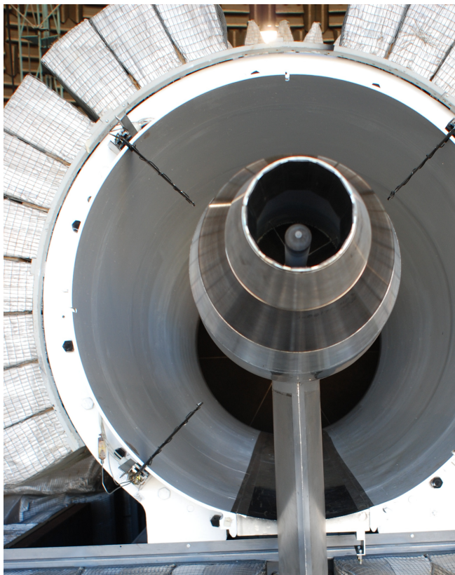
Figure 2.—Photo of the 1/4 th scale F400 nozzle mounted to the High Flow Jet Exit Rig at the Nozzle Acoustic Test Rig at NASA GRC. The nozzle is shown in the baseline (no chevron) configuration.
