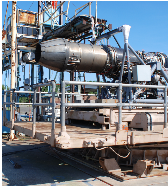
Figure 1.—Photo of the full-scale F404-GE-F400 engine mounted at the Outdoor Test Stand at the Naval Air Engineering Station.
